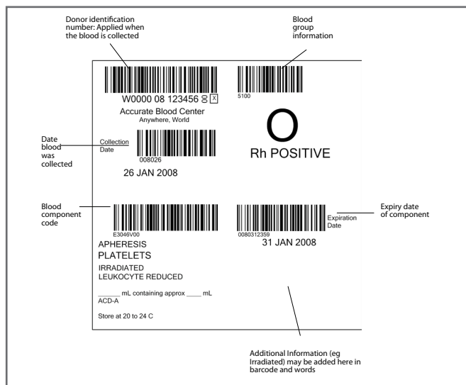
Figure 6.1 International ISBT 128 blood component label as specified in the ICCBBA Standard. www.icbba.org
